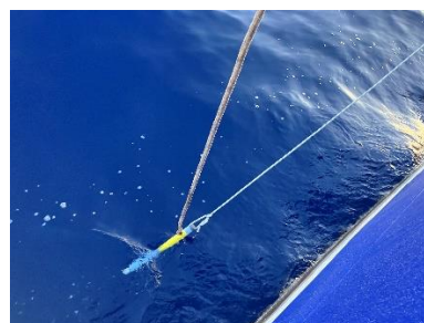
Figure 4: Example of positioning at sea of a hydrophone connected to a buoy
